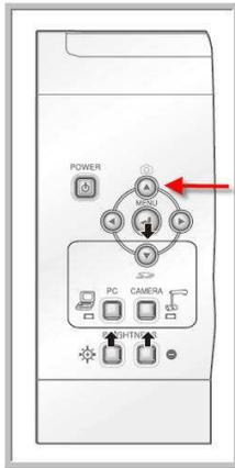
This button (red arrow) is the capture button. Make sure that the On Screen Display (OSD) is not showing on the screen. If it is press the menu button once to turn it off.
